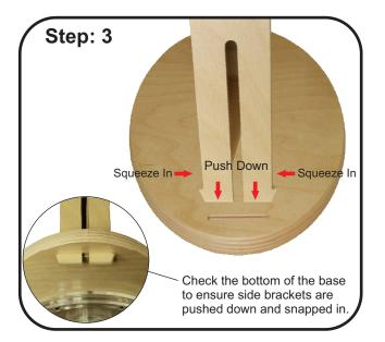
Insert the side brackets in to the base by squeezing the bottom of the bracket while pushing it down into the open slot in the base. Do this for both sides.
